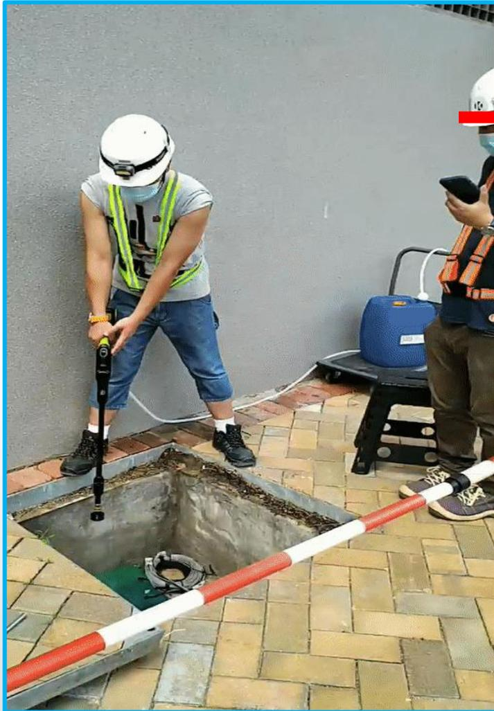
Water blasting to simulate a pipe leak
