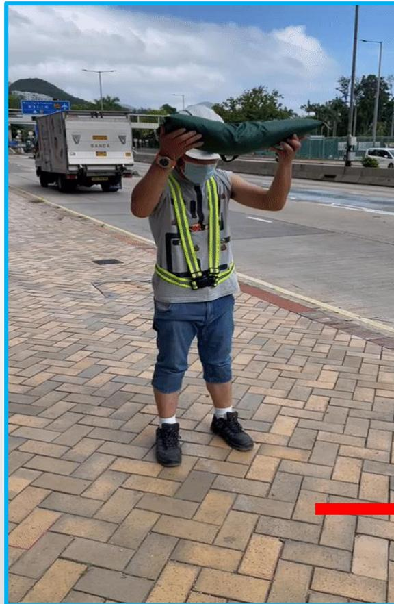
Sand bag dropping to simulate intrusion
