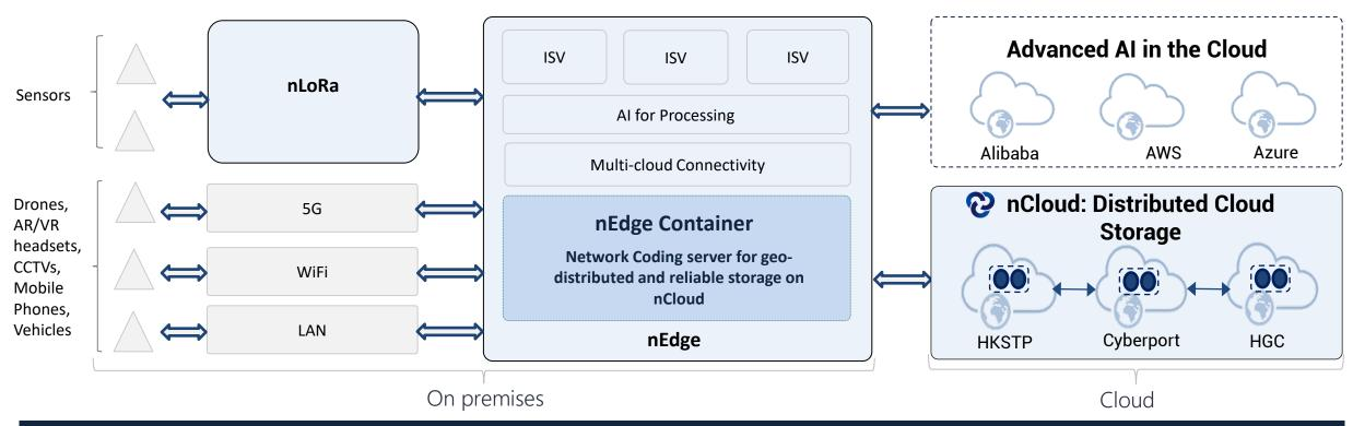
nEdge-nCloud pair leverages multi access technologies to provide computation, communication and distributed cloud storage solution
