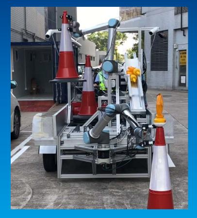
The computer also coordinates the arm operations with the vehicle movement
